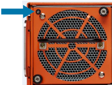
Figure 6 Individual Fan LED Location on GigaVUE-HC3 Rear
